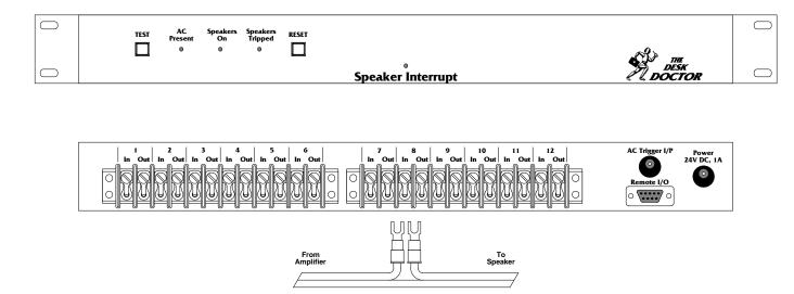
12 Triggerable Relays to Disconnect Speakers from Amplifiers
